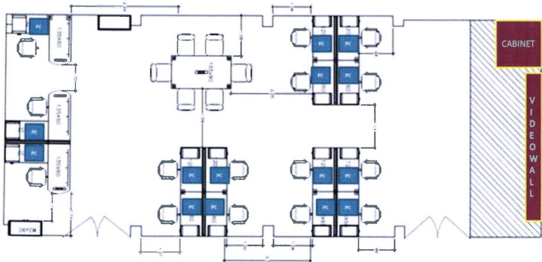
Picture 1. Video Wall Components Location
